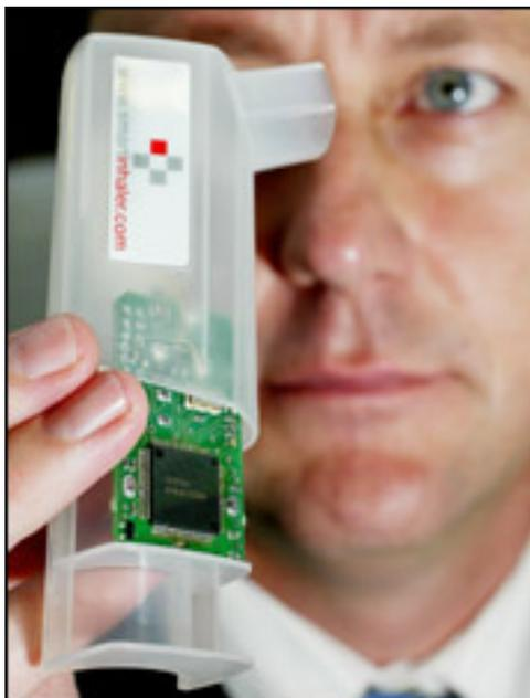
Figure 1 The Smartinhaler™ device
