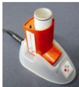
Figure 2 The Smartinhaler™ in its docking station
