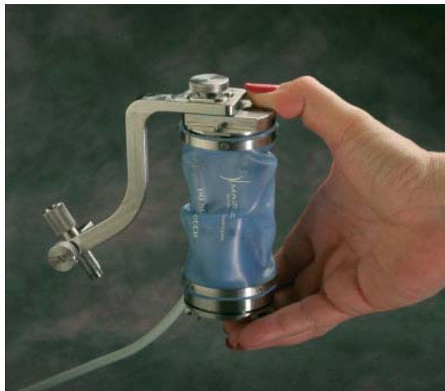
Figure 2: The SpineAssist miniature robot with attached surgical instrument or tool guide. (Source: Sukovich et al 2006)
