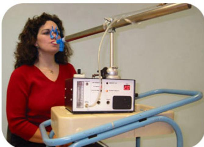
The lung breath test is a non-invasive test that measures volatile organic compounds (VOCs) in exhaled breath to predict the probability of lung cancer. A portable collection apparatus captures the VOCs in one litre of breath into an absorbent trap. The absorbent trap is then analysed by gas chromatography and mass spectroscopy.
